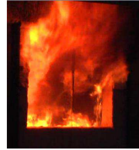
Figure 11. Test PRF-03: All visible combustible surfaces igniting (flashover: 190 – 270 s).
