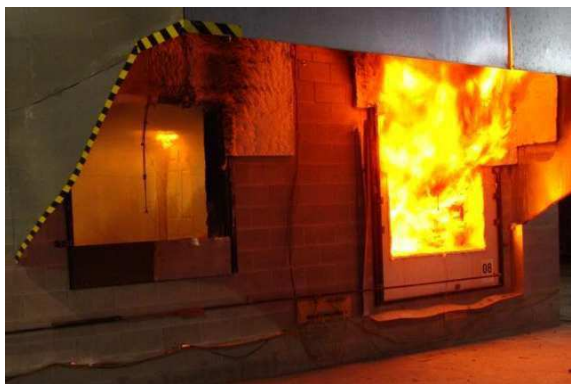
Figure 91. Test PRF-08: Fire starting to burn through the door at 4.5 min.
