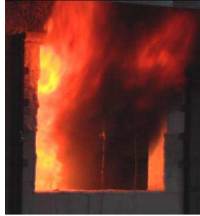
Figure 10. Test PRF-03: Transition to flashover – flames flowing out of entire width of window.
