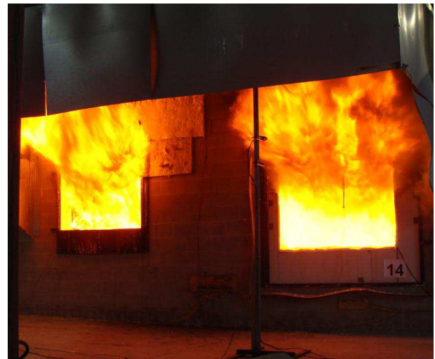
Figure 118. Extent of external burning: flames issuing out of the windows during the post-flashover stage in Test PRF-14.
