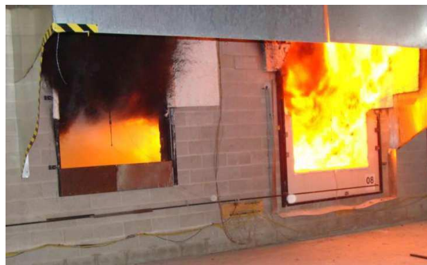
Figure 92. Test PRF-08: Fire burns through the door at 6.5 min.
