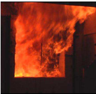
Figure 12. Test PRF-03: Poor efficiency post-flashover (270 – 510s; no visibility inside room).
