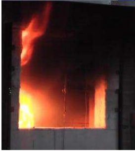
Figure 9. Test PRF-03: Flames flowing out of the top left corner of window (130 – 160 s).
