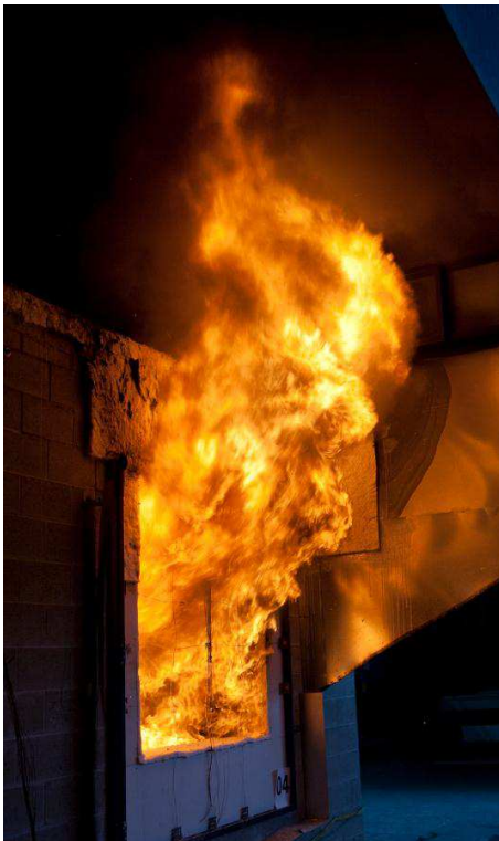
Figure 117. Extent of external burning: flames issuing out of the window during the post-flashover stage in Test PRF-04.
