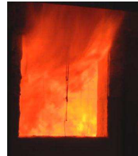
Figure 14. Test PRF-03: Onset of decay phase – flames flowing out of the window with decreasing vigour (inside room becoming visible).
