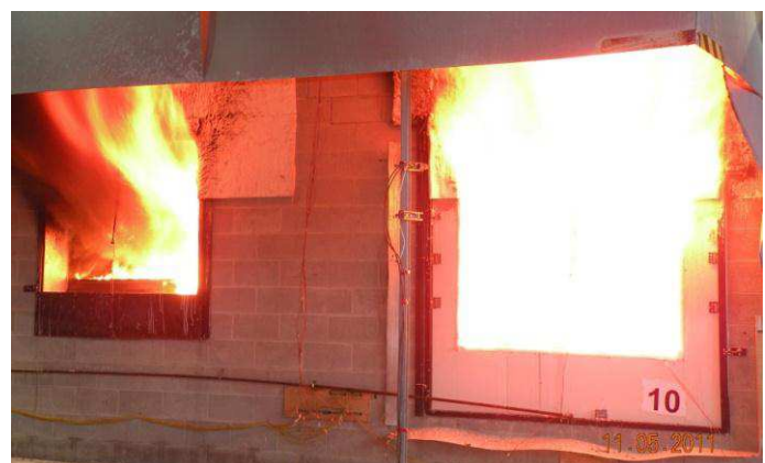
Figure 6. Multiple flashover case (Test PRF-10): Flashover in Zone 2.
