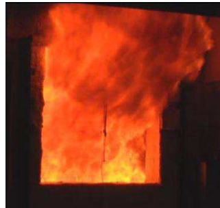
Figure 13. Test PRF-03: High efficiency post-flashover – flames vigorously flowing and extending out of the window (no visibility inside room).
