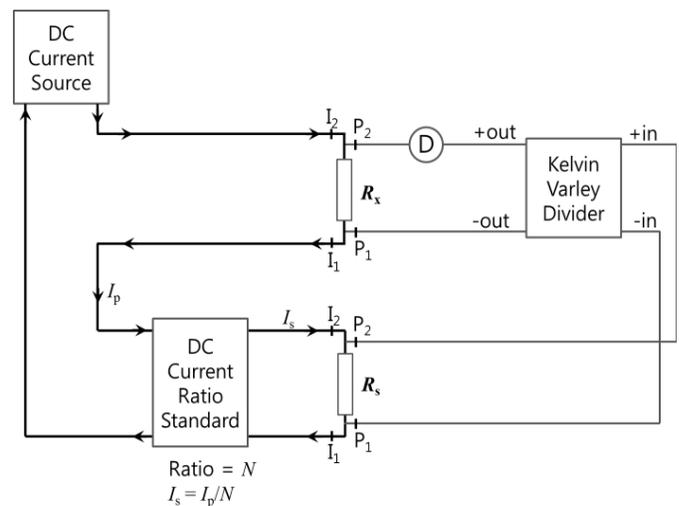
Fig. 3. Calibration of a dc shunt.
