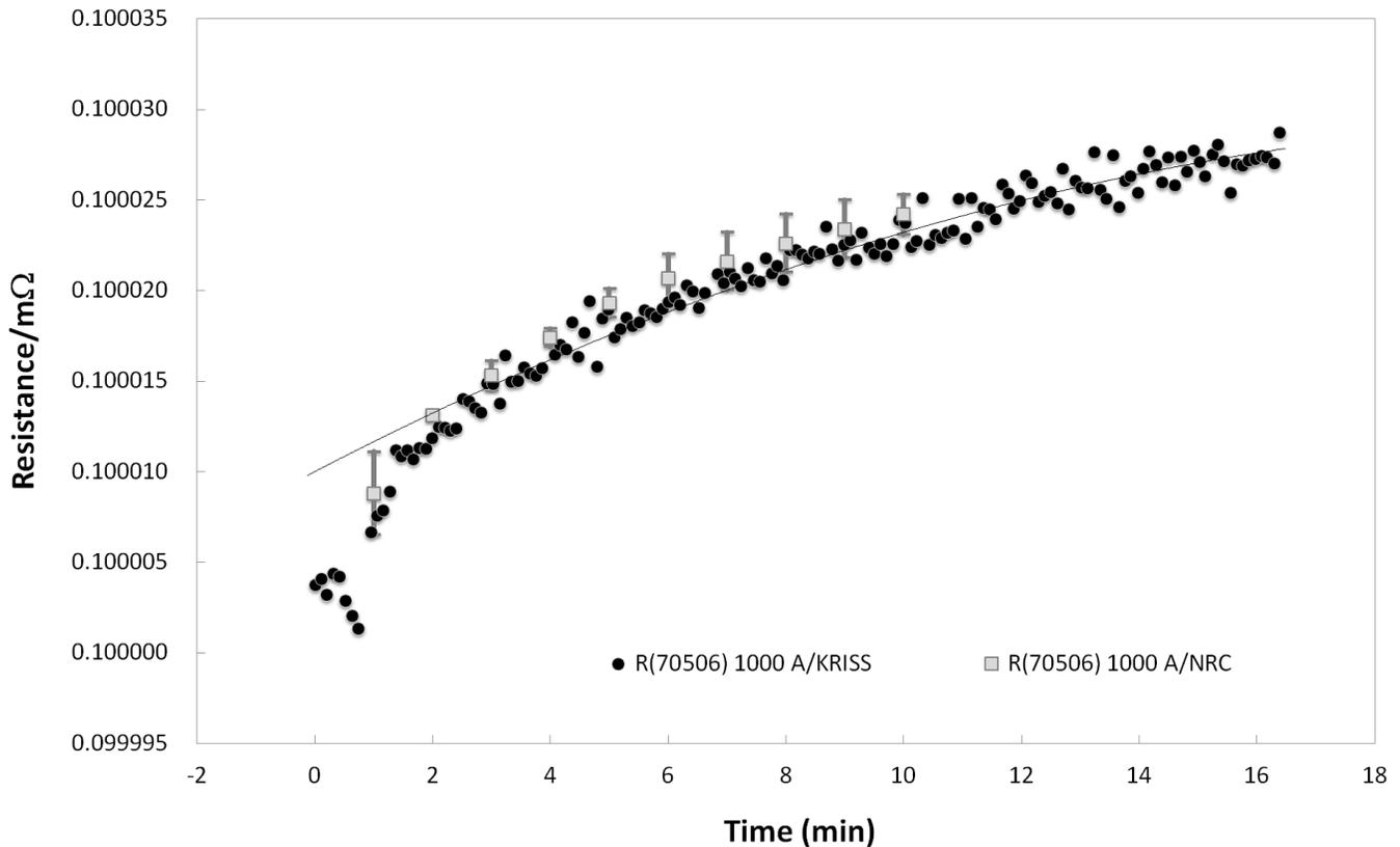
Fig. 2. Shunt-resistance measurement result as a function of time after 1000-A test current applied. The solid circles: the KRISS measurement by the modified step-up procedure. The gray squares: the NRC measurement. The vertical lines on the NRC data represent the two standard deviation margins.
