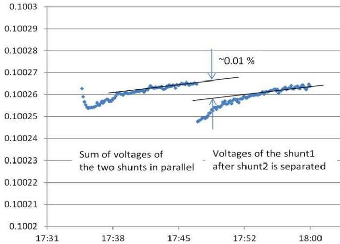
Fig. 1. Voltage readings in volts for the evaluation of the current dependence of the 1000-A shunt during the 500–1000 A step-up procedure [4].
