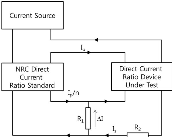
Fig. 4. Calibration of dc ratio device.
