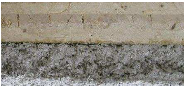
Figure 4: Specimen I-11 with SFRM
