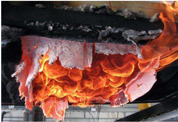
Figure 6: Specimen removal from furnace
