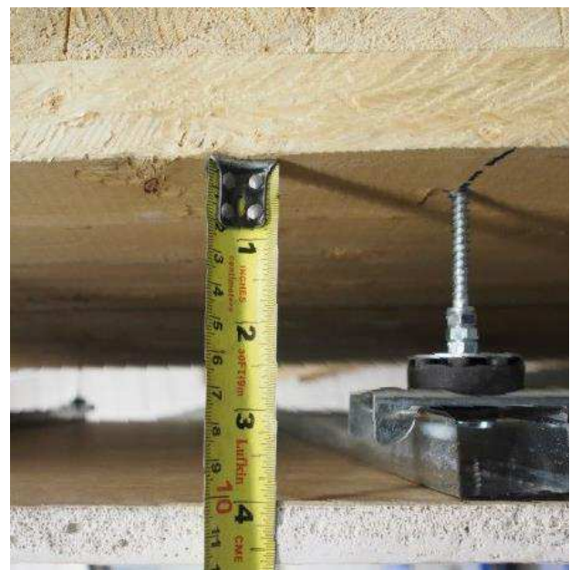
Figure 2: Specimen I-9 with 100 mm cavity
