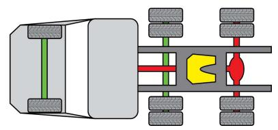
Figure 3: 6x2 pusher tag 6x2 architecture [1]
