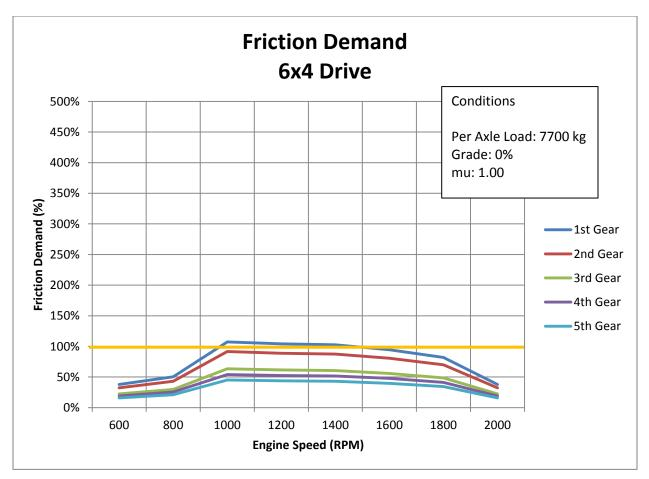
Figure 6: 6x4 friction demand (7,700 kg axle load, 0% grade, mu of 1.00)
