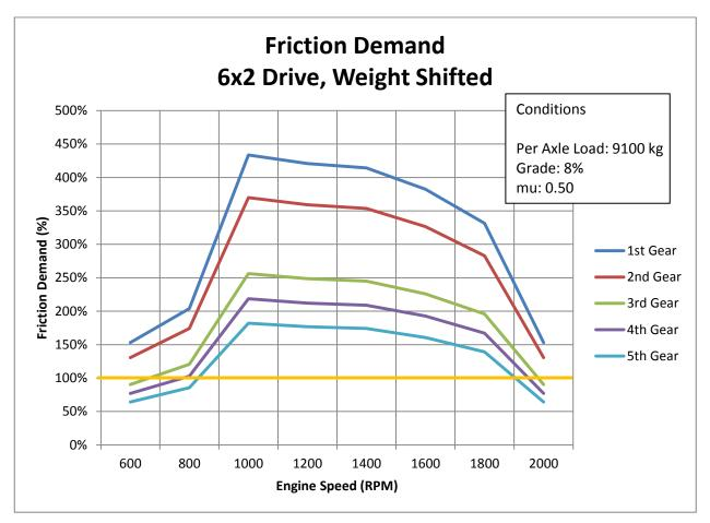
Figure 12: 6x2 friction demand (9,100 kg axle load, 8% grade, mu of 0.5)
