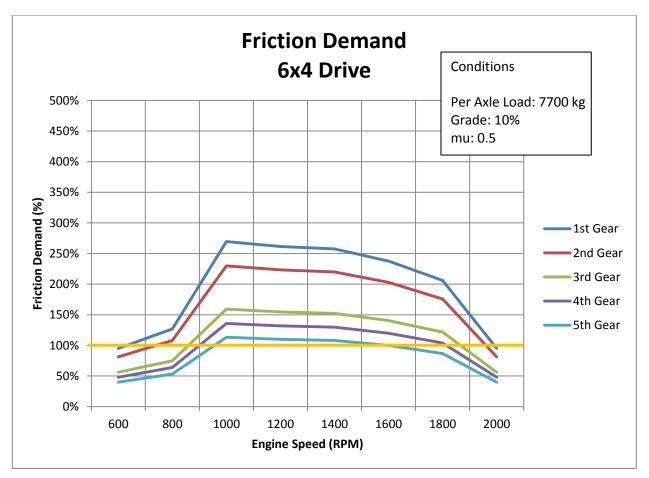
Figure 10: 6x4 friction demand (7,700 kg axle load, 10% grade, mu of 0.5)
