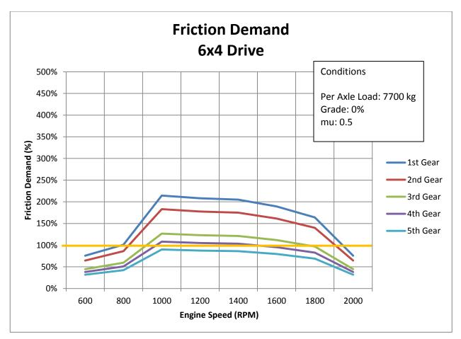
Figure 8: 6x4 friction demand (7,700 kg axle load, 0% grade, mu of 0.5)
