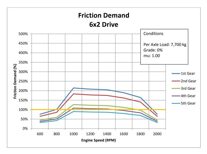
Figure 5: 6x2 friction demand (7,700 kg axle load, 0% grade, mu of 1.00)
