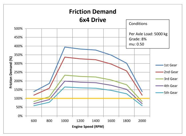
Figure 13: 6x4 friction demand (5,000 kg axle load, 8% grade, mu of 0.5)
