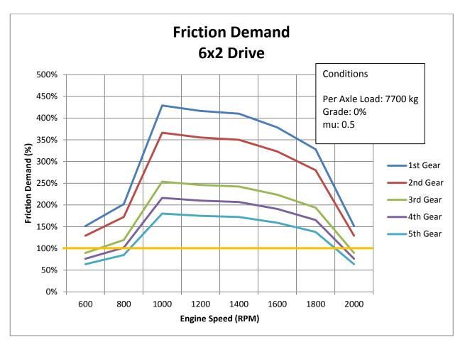
Figure 7: 6x2 friction demand (7,700 kg axle load, 0% grade, mu of 0.5)
