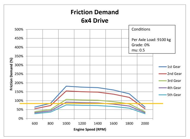
Figure 15: 6x4 friction demand (9,100 kg axle load, 0% grade, mu of 0.5)
