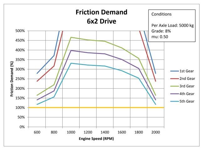
Figure 11: 6x2 friction demand (5,000 kg axle load, 8% grade, mu of 0.5)
