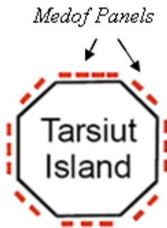
Figure 3-2 Arrangement of 21 Medof panels situated around Tarsiut Island (1982-1983)
