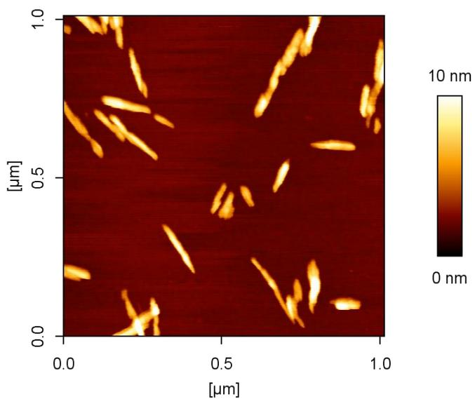
**Figure S2.** AFM image for CNC-RB-1 imaged dry on poly-L-lysine-coated mica.
