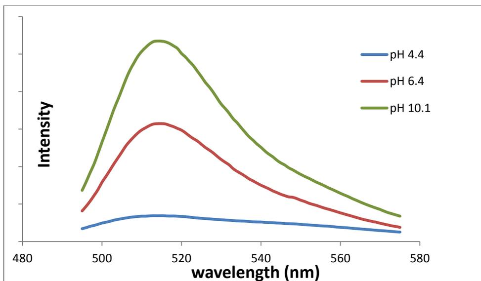
**Figure S1.** CNC-FI fluorescence as a function of pH.
