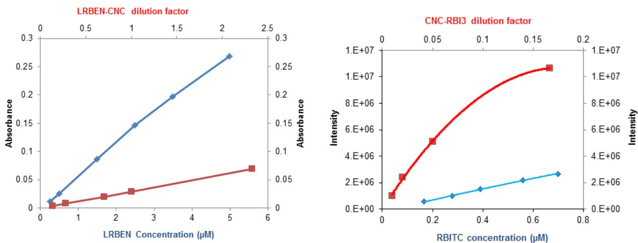
**Figure S3.** (Left) Plots of absorbance vs concentration and dilution for LRBEN and CNC-RB-4, respectively. (Right) Plots of fluorescence intensity vs concentration and dilution for RBITC and CNC-RB-3, respectively. Calculations of fluorescence efficiency were based on the linear portion of the curve.
