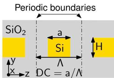
**Figure 1** Cross-section of the sub-wavelength structure. The dimensions are given in table 1 of the main manuscript.
