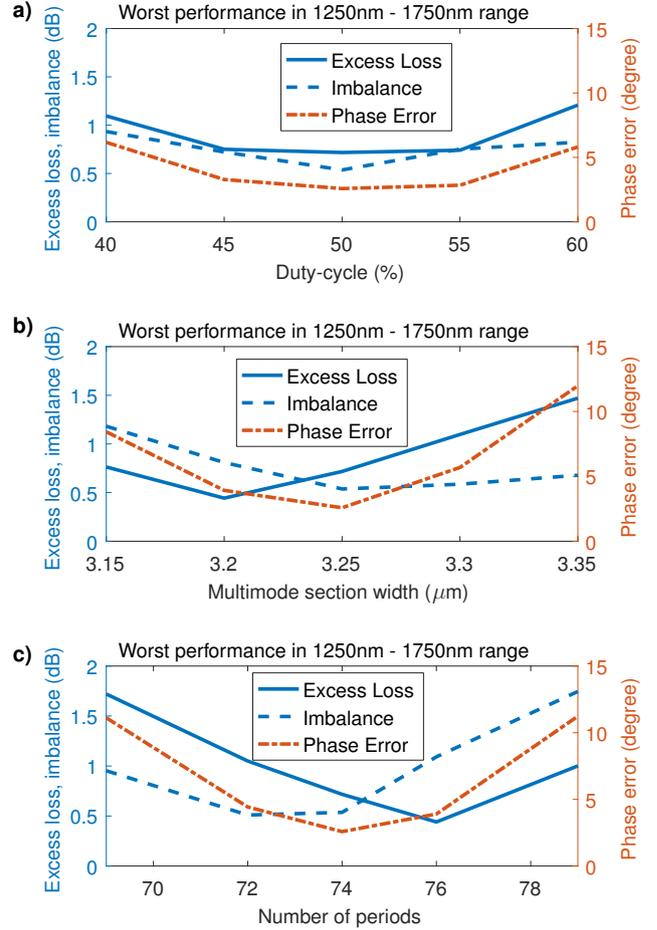
**Figure 3** Simulated worst performance in the 1250 nm to 1750 nm wavelength range, for variations in a) the duty-cycle b) MMI width c) and number of periods, with all other parameters nominal.
