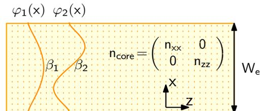
**Figure 2** Multimode waveguide composed of an anisotropic medium.  $W_e$  indicates the effective width that takes into the account the Goos-Hänchen shift at the waveguide walls.
