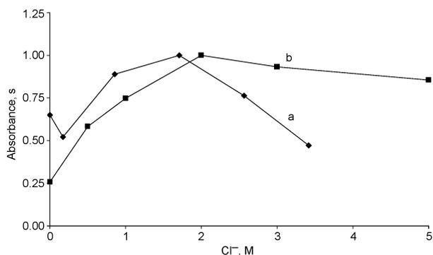
**Fig. 4** Effect of chloride concentration and source of chloride on analytical response: a, 100 ppb TBT in NaCl; b, 20 ppb TBT in HCl.
