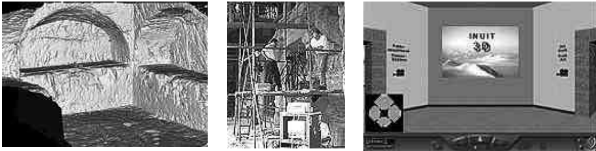
Figure 9. The Tomb of St. James in Jerusalem (left) was scanned using the Large Field of View Scanner in 1996. Note the level of detail captured by the system. One of NRC's industrial partners, Innovision Géomatique used the Biris scanner to scan archaeological sites in China (middle photo). NRC collaborated with the Canadian Museum of Civilization on the production of the interactive web exhibition Inuit 3D for the Virtual Museum of Canada (left).
