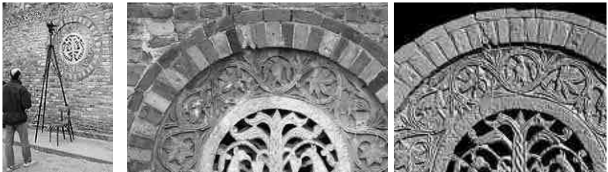
Figure 6. The Biris camera is shown mounted on a conventional tripod (left) scanning a rosone (middle image) on the façade at the 8 th century Abbey of Pomposa near Ferrara, Italy. A photograph of the digital model of the rosone recorded by the system is shown on the right. The digital model records the surface shape and condition of the object after 1100 years exposure to the elements.
