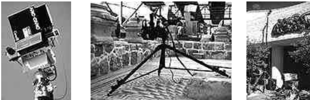
Figure 3. The Large Field of View Laser Scanner (left) mounted on pan and tilt unit. The system includes a video camera to facilitate remote positioning of the scanner. In the center image, the Scanner is shown mounded on a conventional tripod to scan archaeological site features at Caesarea in Israel. On the right, it is shown mounted on a telescoping tripod to scan the sculpture Mythic Messengers at the Canadian Museum of Civilization. The sculpture is mounted 4 m above ground on an exterior wall and measures 9 m long x 1.2 m wide.
