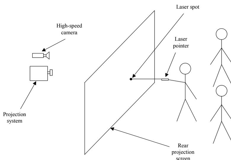
**Figure 5.** Laser-based interaction with wall screen.
