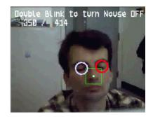
Fig. 6. Using double-blink to switch Nouse on/off.
