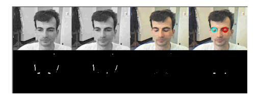
Fig. 4. Detecting eye blinks using the second order change detection. The pixels changed because of head motion removed by the second order change detection procedure are shown at the bottom center images. See also Figure 2.
