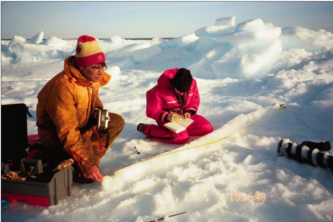
Figure 3-7: Ice Coring and Associated Measurements
