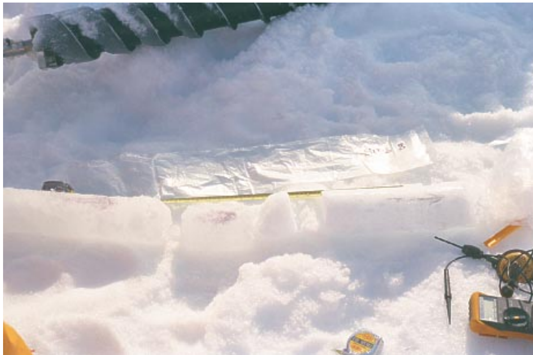
Figure 5-72: Core of Consolidated Layer Retained for Crystallography, Site 8
