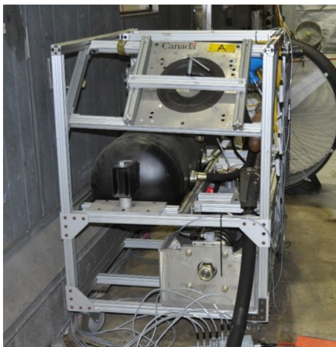
Figure 3. Individual railcar air brake test rig.
