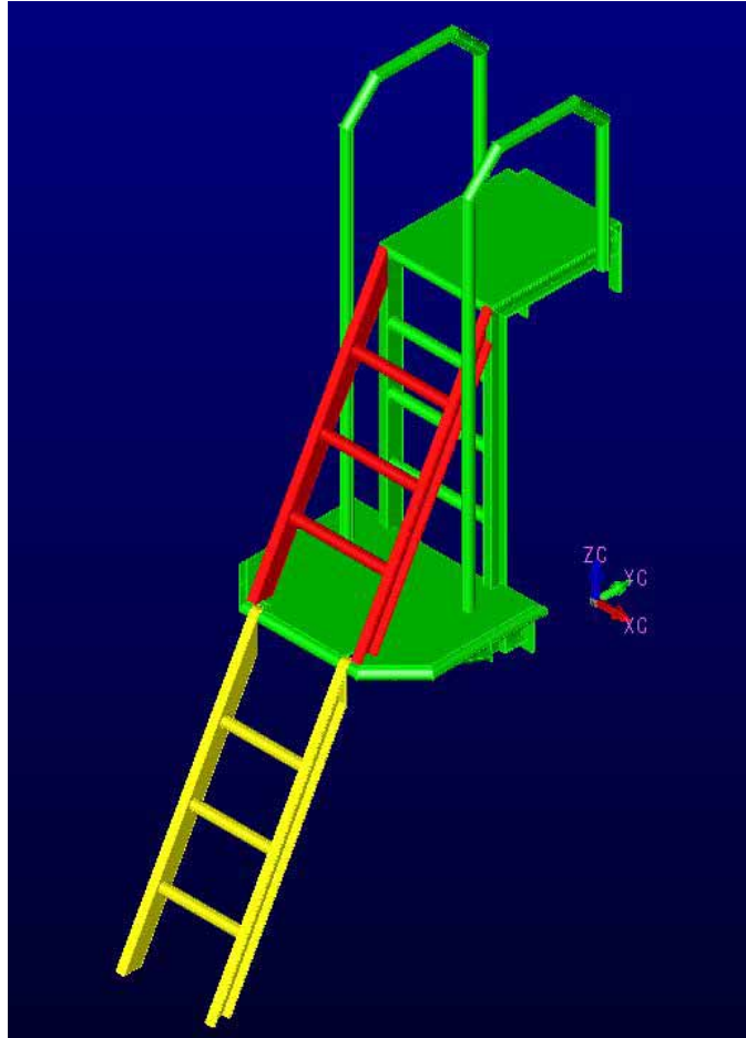
Figure 2: Modified Existing Ladder
